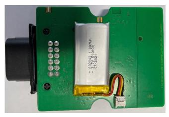
Do not attempt to remove the battery from the cover, once it has been stuck down, as prising or bending could lead to explosion/fire and smoke.
