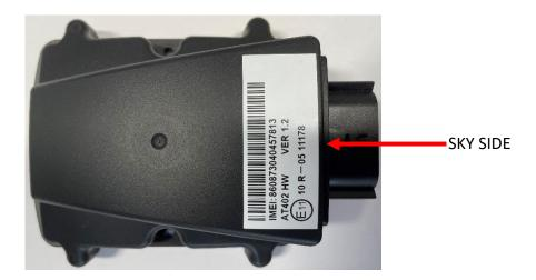
There must be no conductive objects between the AT402 and the windscreen (i.e. nothing metallic, foil or carbon based)
