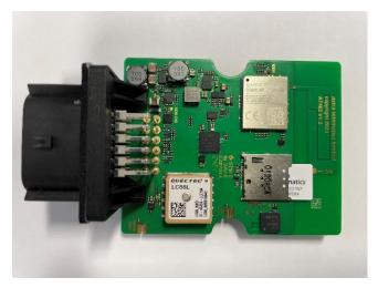
Note that the AT402 powers up when the SIM is inserted
