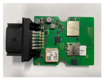
Note that the AT405 powers up when the SIM is inserted
