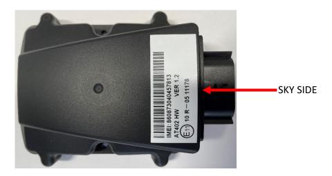
There must be no conductive objects between the AT405 and the windscreen (i.e. nothing metallic, foil or carbon based)
