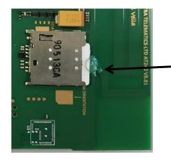
a drop of hot glue can be applied to prevent movement of the SIM, in applications where vibration may cause inadvertent SIM extraction
